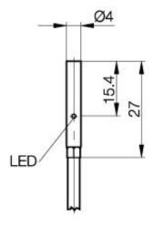
Inductive Sensors BES 516-3018-G-E4-C-PU-02 D4 x 27 normally-closed Sn=1,5mm shielded
